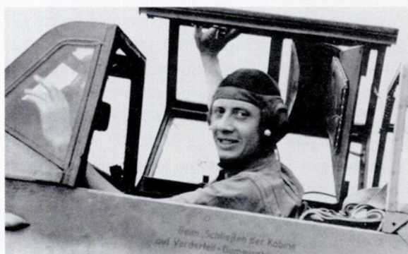
ABOVE: Another photograph of Reinert seated in the cockpit of his Bf 109 G. Note the stencilling under the cockpit sill which reads 'Beim Schließen der Kabine auf Vorderteil-Gummirahmen achten' ('On closing the canopy beware of forward frame seal') indicating that this aircraft had a pressurised cockpit. Only the Bf 109 G-1, G-3 and G-5 had pressurised cockpits.
