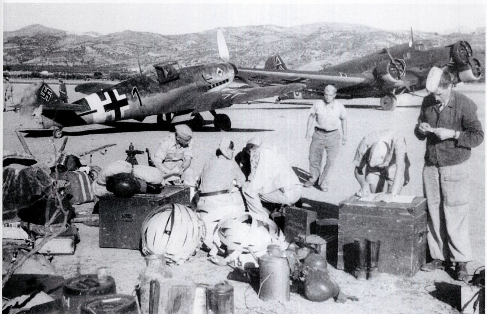
ABOVE: Luftwaffe personnel at Comiso in October 1942 with, behind them, a Bf 109 G-2 of 5./JG 53 coded 'Black 1'. The particularly dark upper surface camouflage on this machine is believed to consist of a brown and dark green scheme applied over the usual RLM 74/75/76 European colours.
