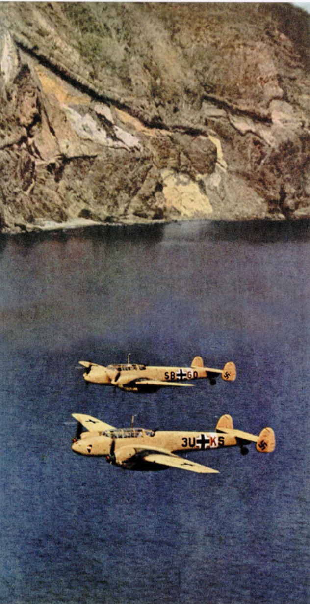
LEFT: A Rotte of ZG 26s Bf 110's on patrol. Both aircraft, believed to be Bf 110 E-2/Ns, are finished in an uppersurface scheme of overall Sandgelb 79, probably with Hellblau 78 undersurfaces. The aircraft in the foreground, 3U+KS, carried the markings of 8./ZG 26, while the second machine still carries the Stammkennzeichen SB+GD.
